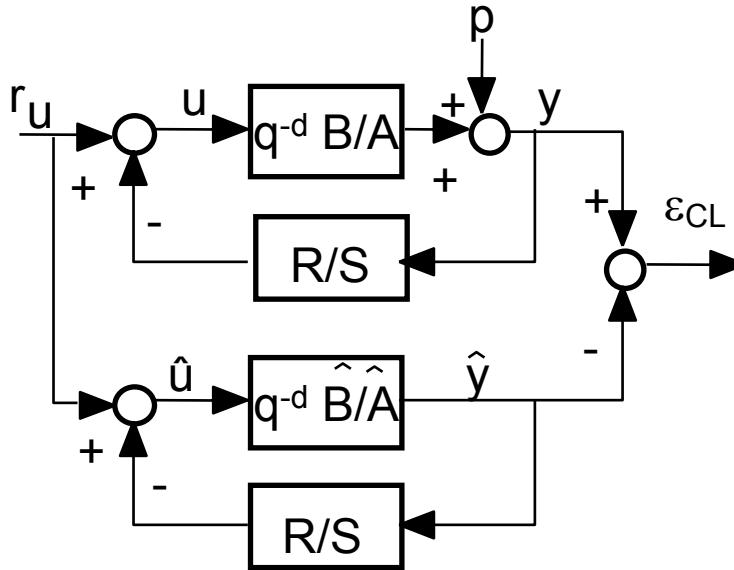
The closed loop system (for  $p = 0$ ):
