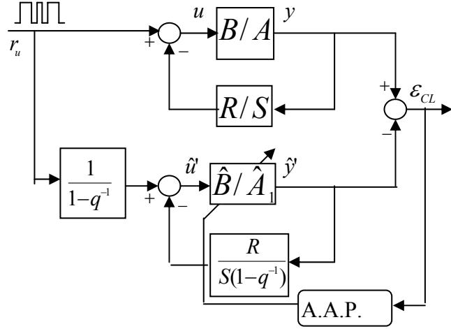
Replace the input of the closed loop predictor by its integral
